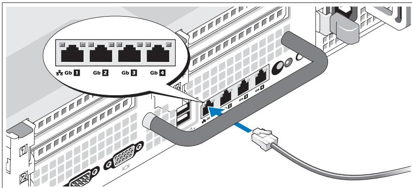
Connect an Ethernet cable to one of the Ethernet connectors at the back of the system.
